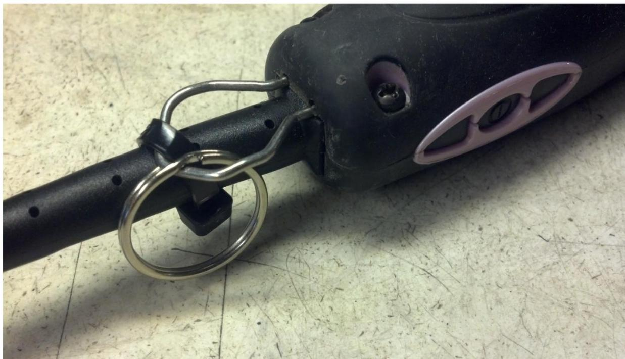
Another issue with this cord, and any other clipper having a voltage converter on the end where you plug it in, is the cord becoming "Dead". These converters, even though they are small, are packed with components. If you accidentally pull this converter out of the wall and it hits the floor, the chances of one of these components breaking is great, thus the cord will become dead, and no electricity will go to the clipper. Below is a picture of the inside of the voltage converter.
