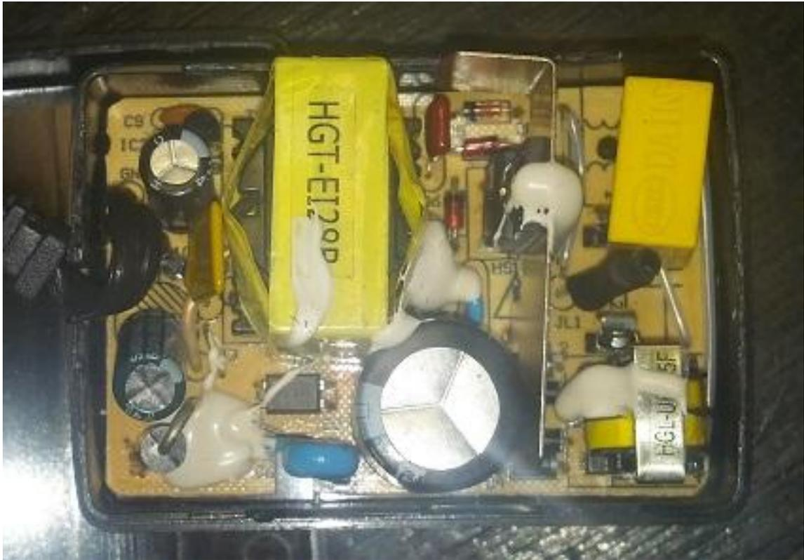
As you can see, there is quite a bit of electronics packed into this small box, and it doesn't take that big of a whack to break something inside if its pulled from the wall socket and it hits the leg on your grooming table. The solution? Get a power strip, and set it on the floor, then plug your cord with the converter into the power strip. It can't fall from the floor, and you just saved yourself the expense of a new cord and sending it off for repairs.
